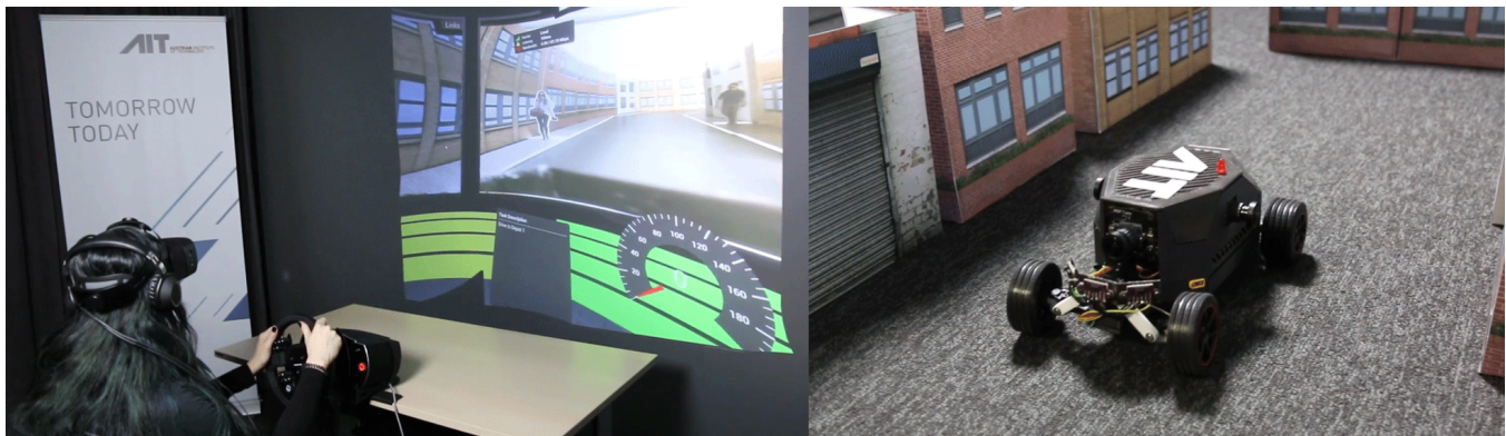
Figure 1: The VR operation station (left) and the vehicle equipped with four 120° cameras and proximity sensors in the physical model environment (right).
