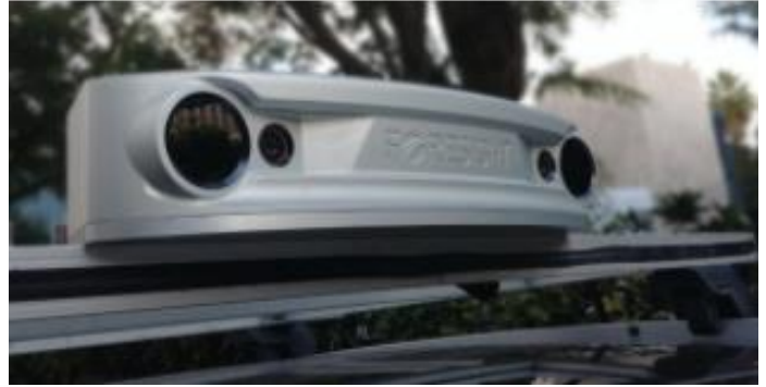
Fig. 1 QuadSight vision system by Foresight ( https://www.foresightauto.com/solutions/quadsight/ )
