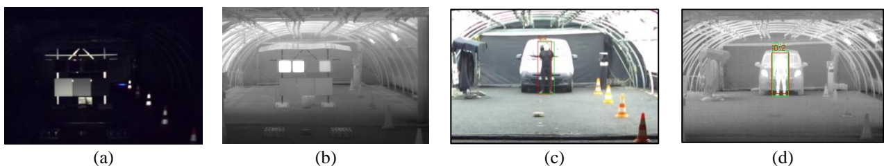
Fig. 3. Presentation of the different targets used during the test. From left to right : Scenario 1 with reference targets, for visible light (a) and thermal cameras (b), Scenario 2 with pedestrian and car, for visible light (c) and thermal cameras (d.)
