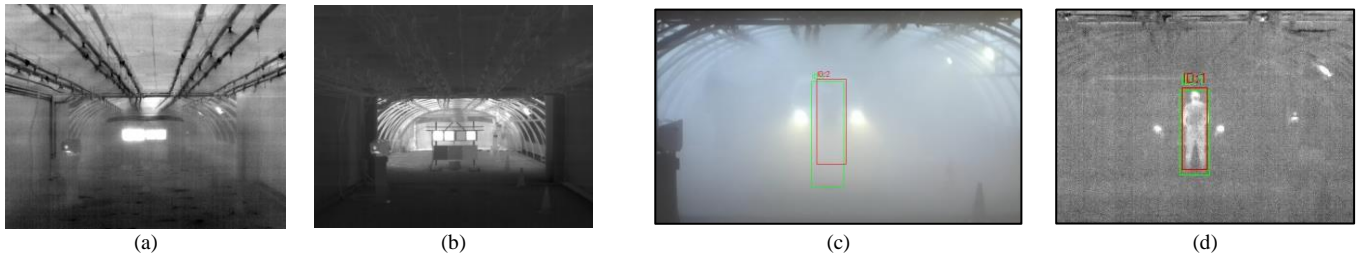
Fig. 5. Different images to better understand the discussion. a. & b. Problem of exposure setup with thermal camera for day and rain conditions (a. wrong exposure, b. correct exposure). c. & d. Example of the pedestrian who is totally invisible on (c.) the visible light camera, while he is perfectly visible on (d.) the thermal camera. Both images (c. and d.) are taken at the same time and under the same conditions.
