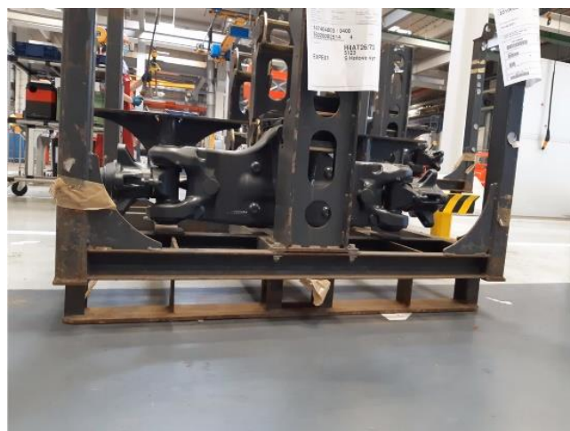
Figure 2. Steering axle rack. Two axles fit on one rack.
