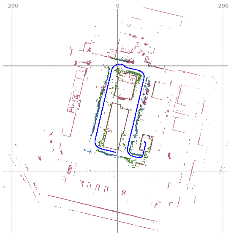
Figure 14: Map generated by Lidars following the blue trajectory, green points (MRS + MCS), red points (VLP32)
