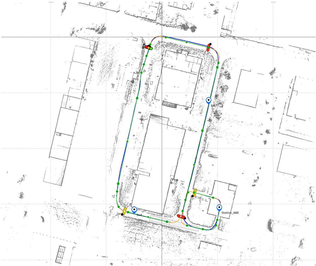
Figure 22: Map generated by the fusion of the lidars for the given path
