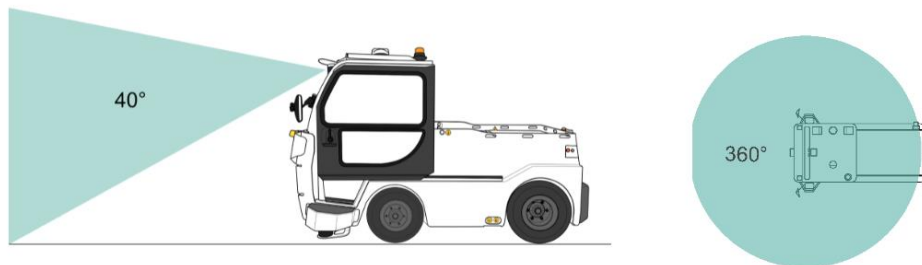
Figure 2: VLP32 Field of View
